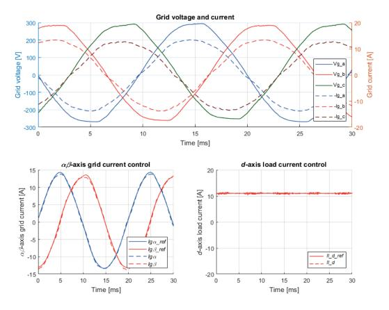
The next figure shows the results obtained using an oscilloscope under the same conditions. As it can be seen, all signals are in phase with the grid voltage and show a low level of distortion.
