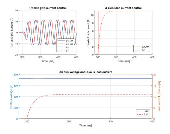
The following figures plot the grid and load currents, respectively (phase A). The load current is filtered through a basic LR-type filter, while the grid current is filtered by a LCL-type filter. The load current ripple reaches 1.7A at this operating point. The grid current ripple is significantly lower and reaches the design value of 10mA.
