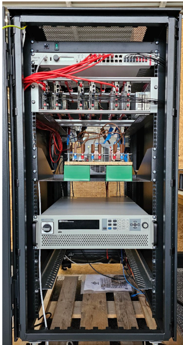
Figure 5: The OBC demonstrator fitting neatly into a cabinet
