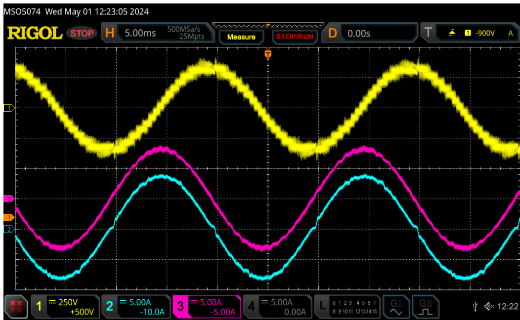
Figure 5: CH1 (yellow) generated converter voltage in phase A, CH2 (cyan) STATCOM converter current in phase A ( I_{s,a} ), CH3 (magenta) load current in phase A. Taken at 1.05 s in Figure 4.
