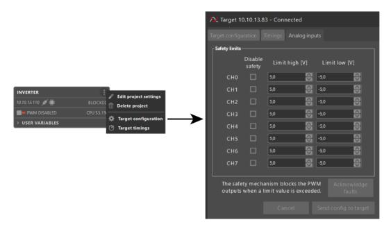
The selection of suitable limit values used as protection thresholds is always a function of the application. It is generally recommended to select limits that are slightly above the planned
