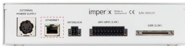
Location of the ethernet port on the rear side of the B-Box Micro
