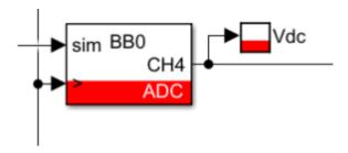
The probe "Vdc" is connected to the output of an ADC block
