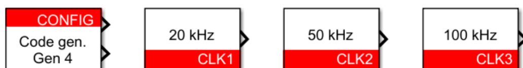
Figure 2 : Configuration blocks for the four different clocks (The displayed values are only for the sake of example)
