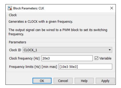
A CLK block using *CLOCK\_0* is already embedded in the CONFIG block. See <u>CONFIG – Interrupt</u> <u>configuration</u> to learn more.
