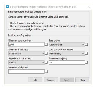
The Ethernet IP addresses can be configured in the Imperix Controllers' target window (Coder → Coder option → Target).
