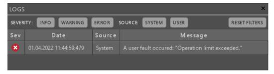
To stop the system in case of abnormal operating conditions, it is advised to rely first and foremost on the hardware protection mechanism of the B-Box RCP, when possible. Using the user fault block and software comparators for that purpose leads to a longer response delay and a lower level of safety.
