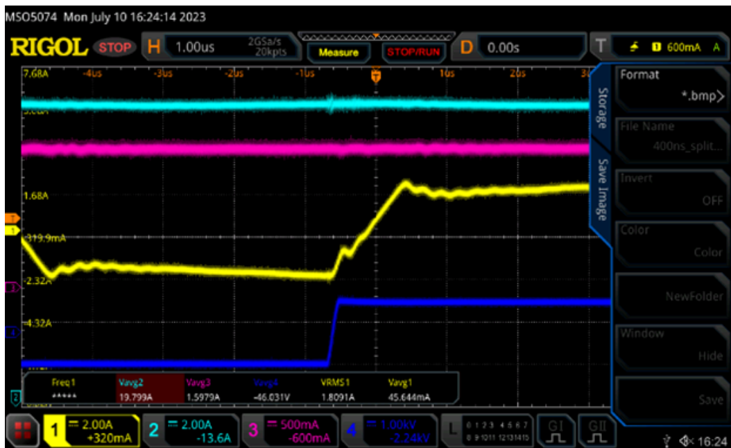
DAB waveforms with split inductors on each primary leg
