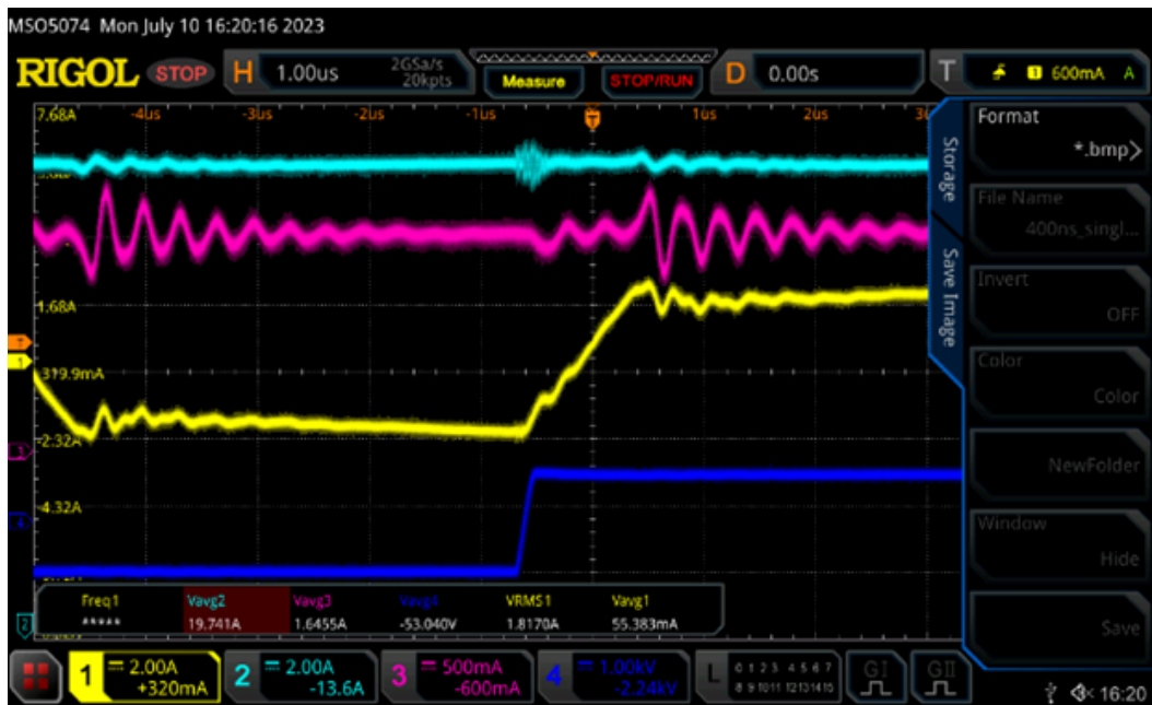
DAB waveforms with single external inductor
