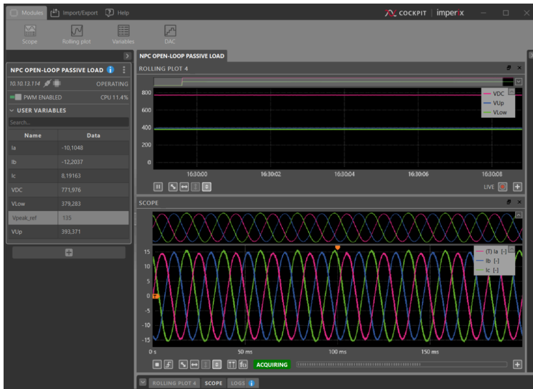
Fig. 11. Cockpit session with 0.8 as modulation index, 120V on the DC bus and enabled PWM.
