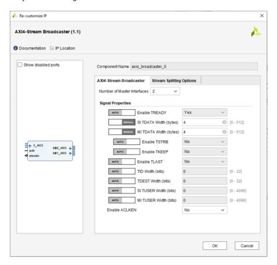
**WARNING 1:** Note that users should not leave the output ports floating or not connected to a AXI4-Stream slave. Since the AXI4-Stream Broadcaster IP doesn't provide a default *tready* signal, a floating output port will block the dataflow. A relevant discussion about the problem caused by floating *tready* is in <u>Solved: axis broadcaster – Community Forums (xilinx.com)</u>
