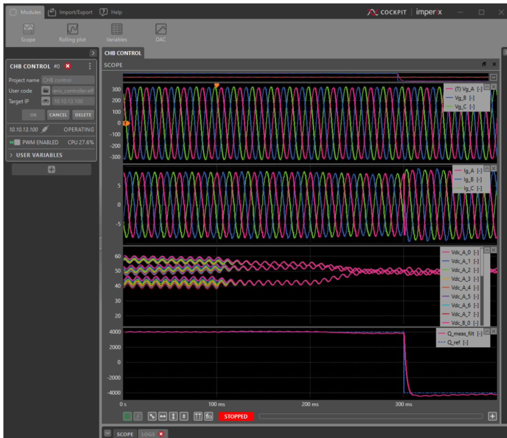
Figure 7: Experimental results for the grid-connected cascaded H-bridge with N=24 H-bridges showing the effect of balancing and a reactive power step response
