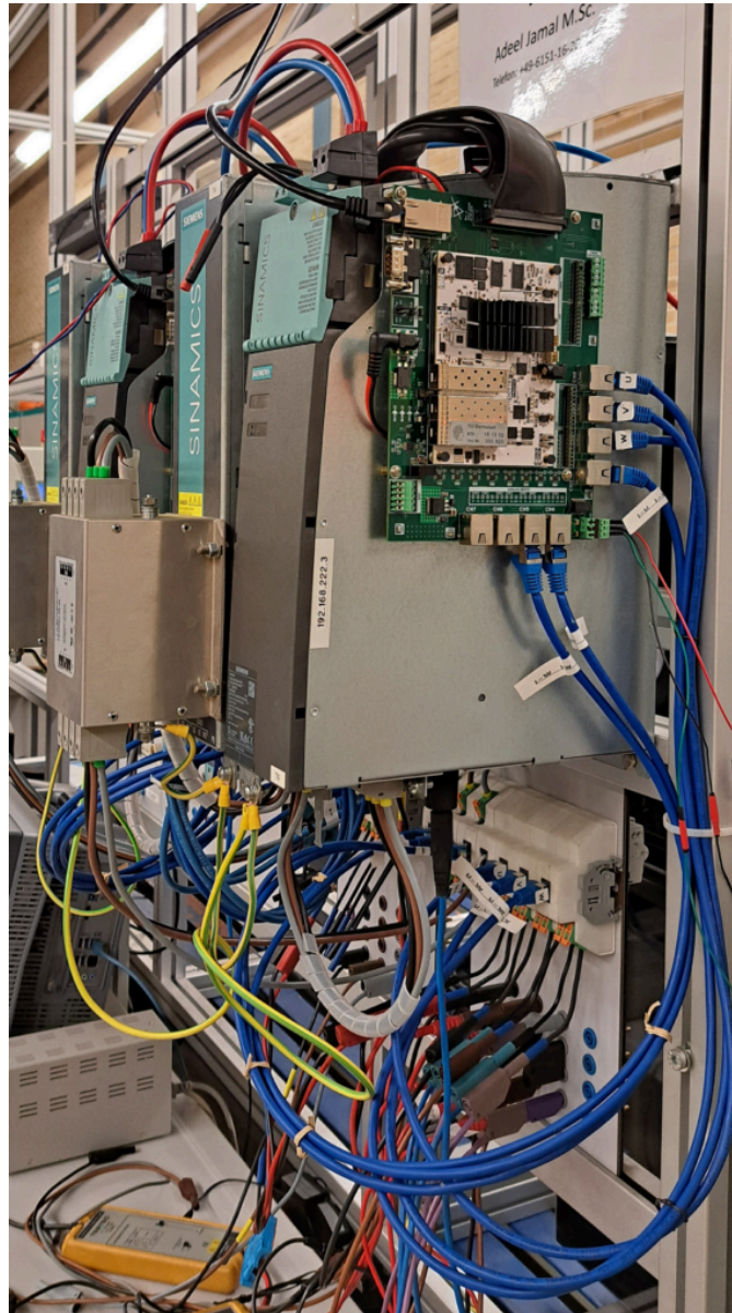
Figure 1: B-Board PRO mounted on the carrier board and external imperix sensors connected
