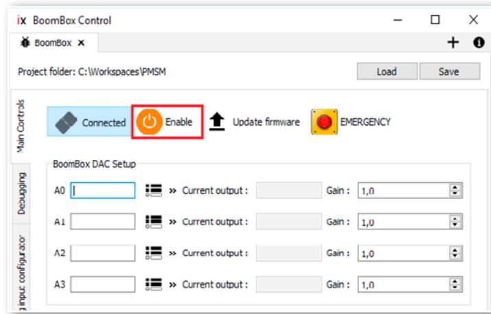
The enabling/disabling process is independent from the control algorithm running on the BoomBox and acts as a switch on all PWM signals :
