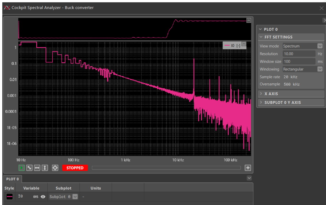
FIGURE 2 : SPECTRRAL ANALYZER MODULE SHOWING THE FFT OF A CURRENT WITH ITS SWITCHING HARMONINCS.
