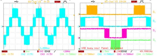
Figure 3: Generated output voltage at no load (left), as well as the corresponding PWM patterns (right).
