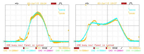
Figure 3: Performance evaluation comparing the estimated value with the actual measurements. (a) current Id12, (b) current Id11
