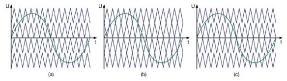
Figure 2: 5-level modulation approaches. (a) PD, (b) APOD, (c) POD.
