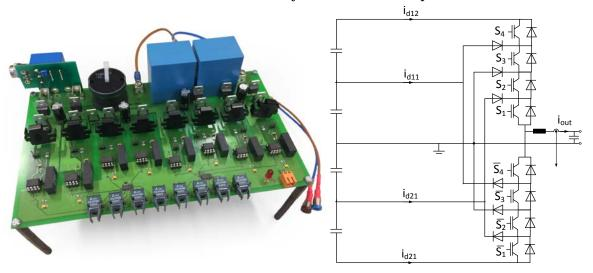
Figure 1: Photograph and schematic of the studied 5L-NPC converter topology.
