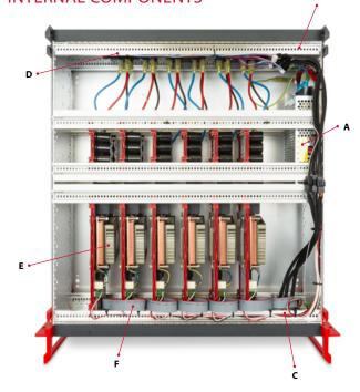
Type C enclosures can host different types of modules, which are commercialized as independent products. One is here shown with 6x PEB8038 half-bridge modules (not included).
