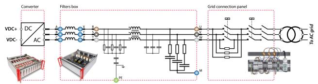
*Figure 10.* Filter topology for a connection to the grid with an isolation transformer.
