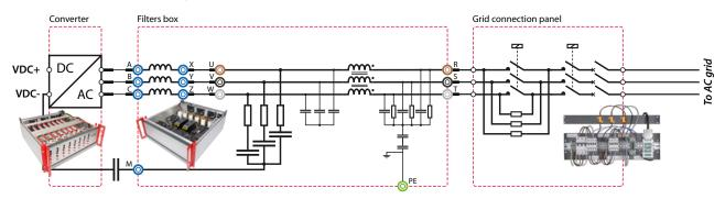
*Figure 11.* Filter topology for a transformer-less connection to the grid.
