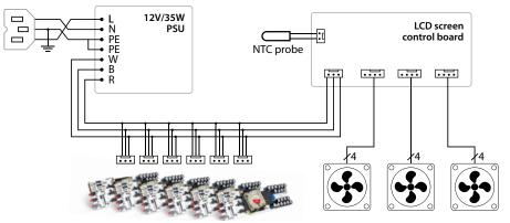
Figure 9. Electrical schematic of the auxiliary circuit.
