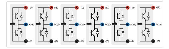
Figure 1. Electrical schematic of the main power section, corresponding to the individual power modules.
